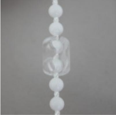
The correct position of the breakaway device is just below the chain drive, on the down side of the chain, when the blind is fully up. This ensures that the operating load on the chain breakaway device is the least possible because the weight of the blind is working with the breakaway device.
