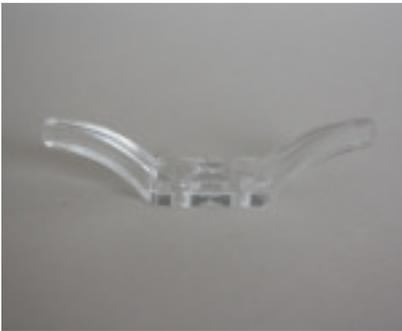
The safety cleat must be installed no lower than 1.5 metres to the floor, as close to the headrail as possible and the cleat must be able to take all of the cord when the blind is fully up. If one cleat cannot take all of the cord install two cleats, one above the other, approximately 15cm apart or sufficiently apart to ensure that all of the cord can be accumulated on the cleats and no part of the cord or acorn is lower than 1.5 meters to the floor.
